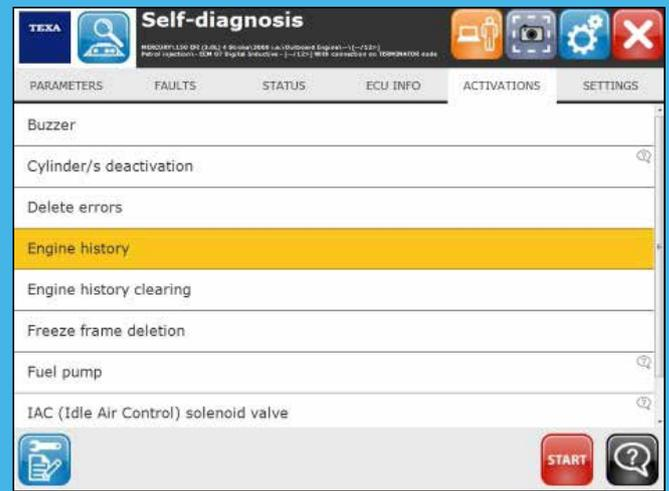
3. Navigation within the software screens is easier thanks to the use of tabs (PARAMETERS, STATUSES, ERRORS, ECU INFO, ACTIVATIONS, ADJUSTMENTS).
