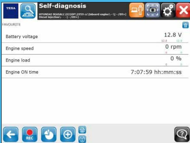
4. Favourite buttons with Print, Recording, Deletion and function buttons: FREEZE FRAME, Self-diagnosis Help, component wiring diagram and solved problem service.
