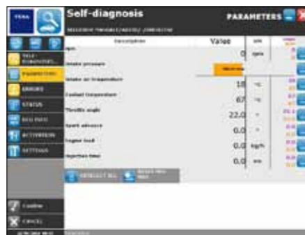
Remote diagnostics of fuel injection control unit and parameters.
