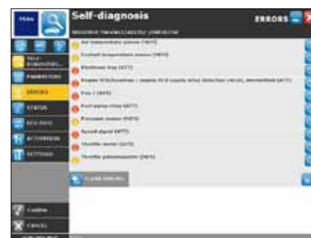
Reporting of errors logged in fuel injection control unit.
